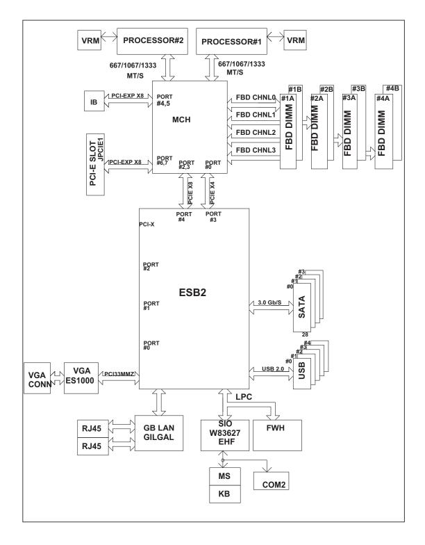
Figure 1-1. Intel 5000P Chipset: System Block Diagram
